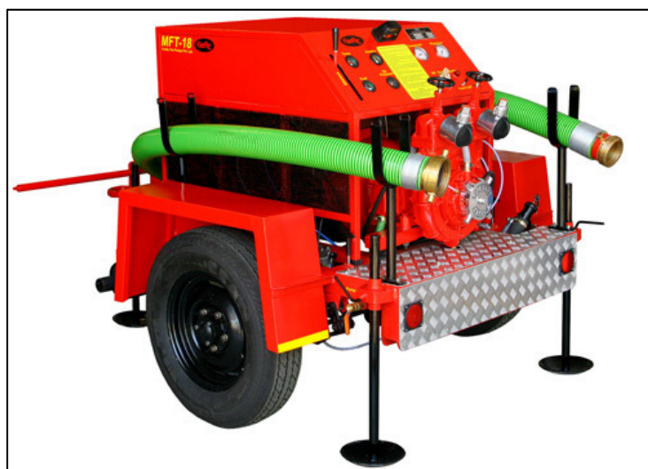
Fig 3. Example of Trailer Pump suitable for water transfer with tank fill capability.
