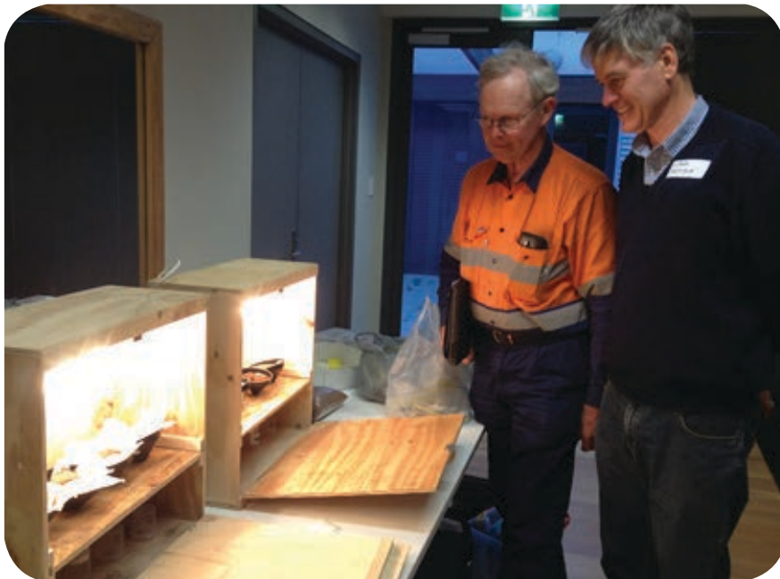
Figure 7 Tullgren Funnel apparatus for extracting soil fauna in a Light Box. The Men's Shed in Northam, WA built these 'light boxes' for use by farmers within the Wheatbelt NRM region (Photo: L Abbott; Leibe Group Workshop).
